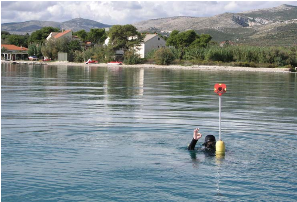
Figure 5: Recording the corners of the grid by a total station (Photo by author).
