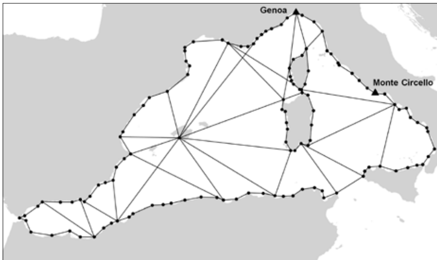
Fig. 1 Geodetic framework of distances and azimuths between coastal points in the Western Mediterranean. Similar frameworks were defined for the Eastern Mediterranean and the Black Sea. Calculation or plotting of the positions of the coastal points yields a 'synthetic' chart that can be compared to a portolan chart.
