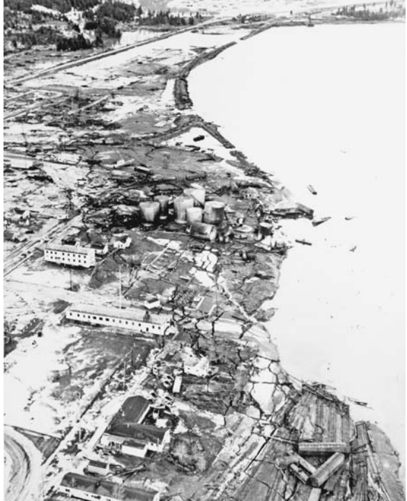
Aerial view of Seward after tsunami, showing destruction of waterfront and curved scalloped shoreline formed by submarine slumps removing several blocks from the shoreline ( University of Alaska Fairbanks )
