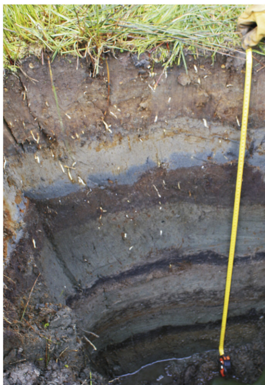
Fig. 7. Maullín, Chile: a series of stacked tsunami and palaeotsunami deposits topped by the 1960 AD event (photo: J. Goff). Interestingly, while there is a direct historical association between subduction zone earthquakes and tsunami inundation in the region, little proxy work has been carried out on the prehistoric sediments. One of the lower events is also believed to be an orphan tsunami from a more distant palaeosource (refer to Cisternas et al., 2005 for details about this area).
