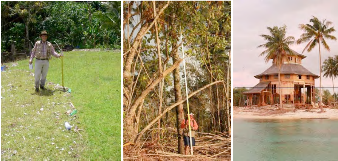
Figure V-8: (left) A clearly identifiable tsunami trace in American Samoa, 2009 (mid) Indicators of tsunami flow depth are less clear in this example from the Mentawai Islands; note the broken branches and (right) flow depth indicated on a photograph by an eyewitness.
