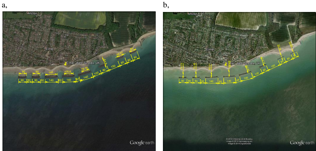
Figure 3.13: The tombolo measurements at low water level (a) and the salient measurements at high water level (b) at Elmer, the UK
