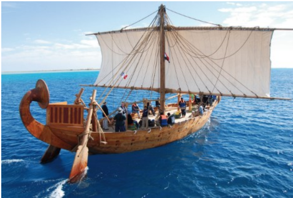
Figure 6: Min of the Desert is a reconstruction—a synthesis of archaeological data drawn from excavated timbers and hulls, along with representations and models—as no seagoing Egyptian ships have been located. Photograph courtesy of S. Begoin.
