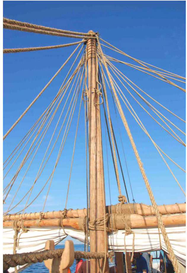
Figure 17 b: Rigging arrangement
