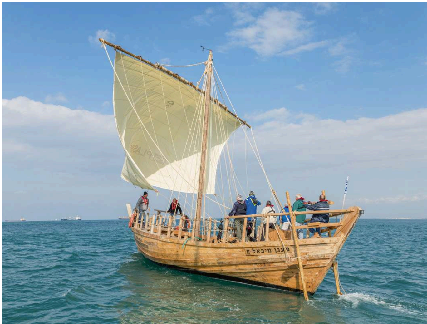
Fig. 3: The Ma'agan Mikhael II under sail on a broad reach. The two quarter rudders can be seen (photography E. Efremov).
