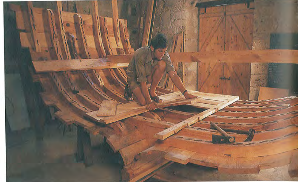
Left Fitting outer planks together over close-spaced tenons, shipyard owner Manolis Psaros (below) and master shipwright Michaelis Oikonomou of Perama, Greece, recreate ancient shell-first construction.
