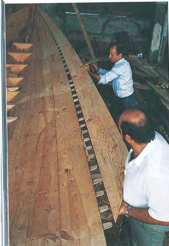
Left Fitting outer planks together over close-spaced tenons, shipyard owner Manolis Psaros (below) and master shipwright Michaelis Oikonomou of Perama, Greece, recreate ancient shell-first construction.
