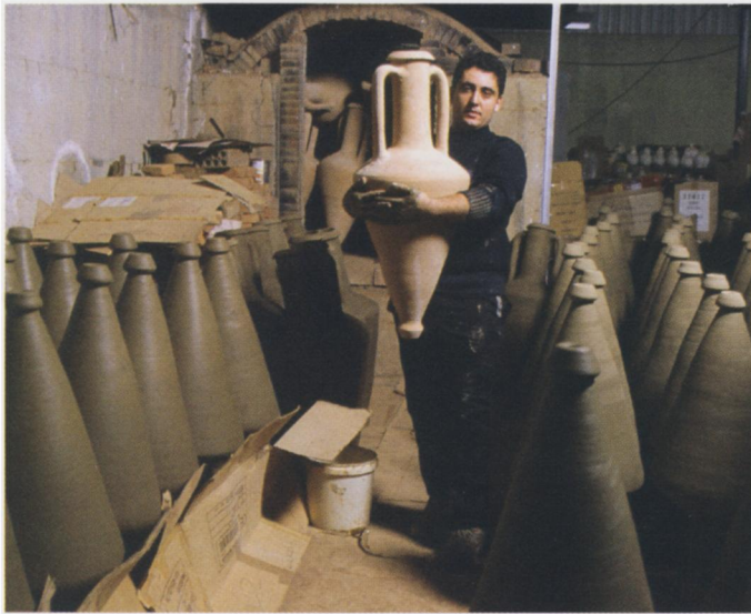
An "army" of inverted Rhodian amphorae flanking Nikos Pandeis waits to dry. He holds one just out of the wood-fired kiln behind him. The Pandeis family restored this kiln, long in disuse, to recreate the Kyrenia Ship's cargo. Photo by Radomir Cvetic.
