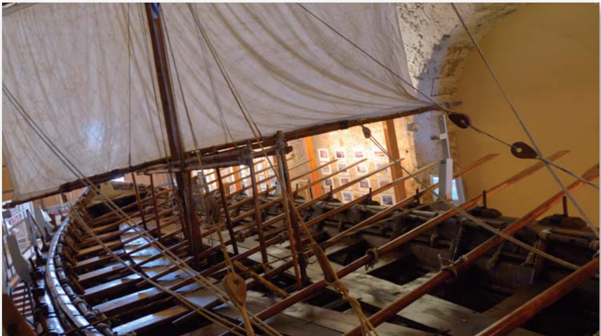
A reconstructed Minoan vessel, now in the Maritime Museum in Chania, Crete, showing the sail footed with a boom, a distinctive feature of many Minoan ships. The gangway is mounted upon the rowing benches, providing height during boarding actions. Note that in the absence of dedicated storage, the oars are laid across the gunwale. (Alamy)
