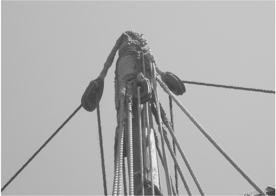
Figure 2-7. Masthead blocks on the Kyrenia Liberty replica. The central block is one of two halyard blocks, while the blocks on either side are carrying the lifts supporting the yardarm (Photo: J.Whitewright).
