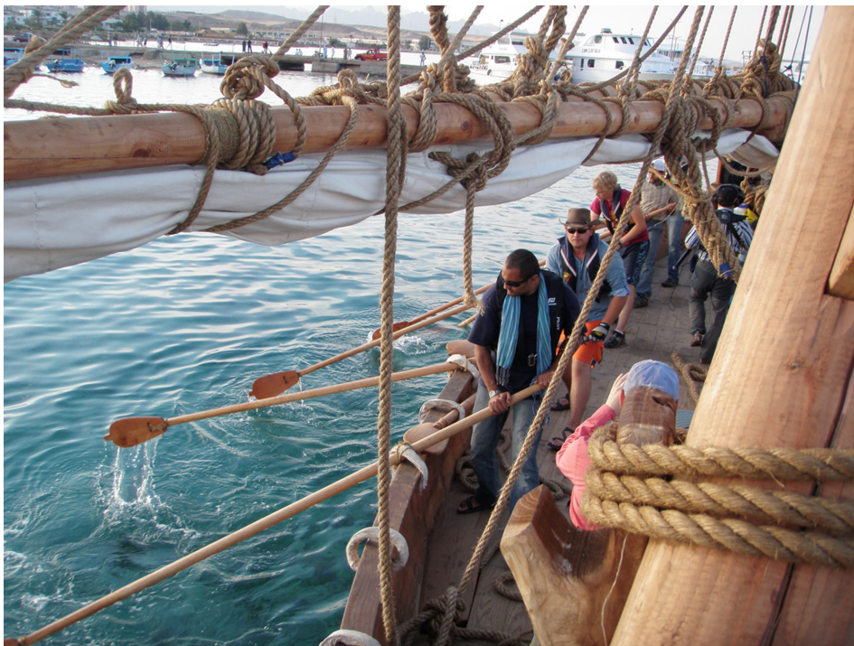
Fig 8: Rowing provides speed enough for maneuvering the ship in and out of anchorages, but was unlikely to be a primary propulsion means for the ancient Egyptians at sea.
