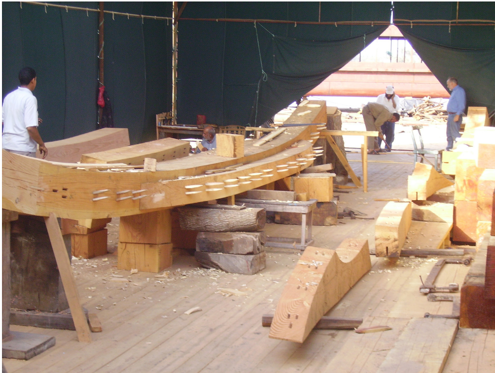
Fig. 1: The wood-to-wood, mortise-and-tenon fastening has a demonstrably indigenous origin in Egypt and was the primary fastening for seagoing ships of the Middle Kingdom. A trapezoidal slip of wood (tenon) is cut to fit tightly at its centre in a pair of mortises that are placed opposite each other in adjacent planks.
