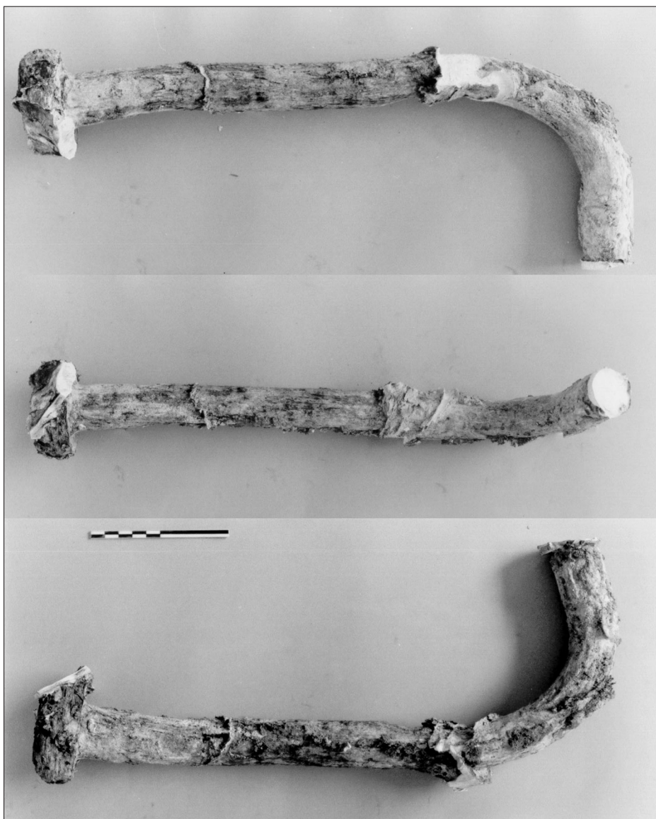
Fig. 7.25. Three views of cast of bolt Q2/C7(V) joining keel and keelson. (Photos Pedro Gonçalves, CNANS; used with permission of CNANS)
