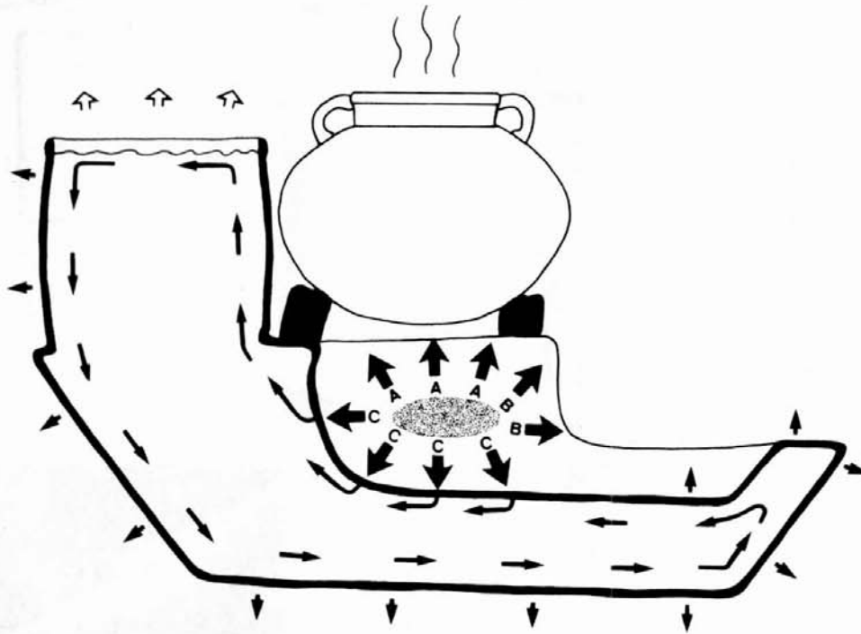
Principle of the Thermo-dynamic System and Water Circulation in a lead brazier
