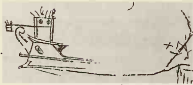
74 Prow of a warship equipped with a fire-pot. A fighting tower stands in the bows and, at the end of a pole projecting from it over the prow, hangs a pot full of blazing fire. Graffito on the wall of a tomb in the Anfushi Necropolis, Alexandria, 1st century BC.
