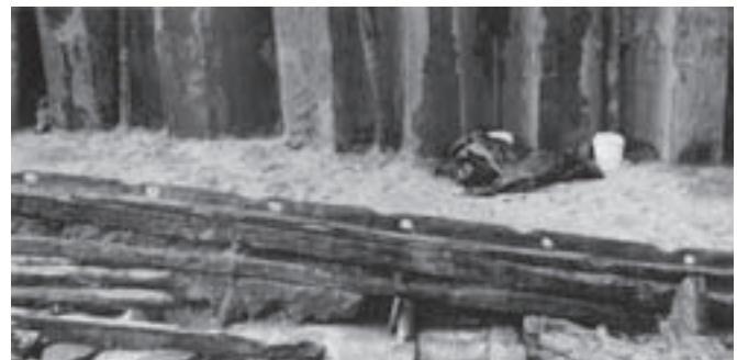
Fig. 9. Rowing fittings of Woerden 7 : gunwale with holes and oarlocks. (after Blom, Vos 2008).
