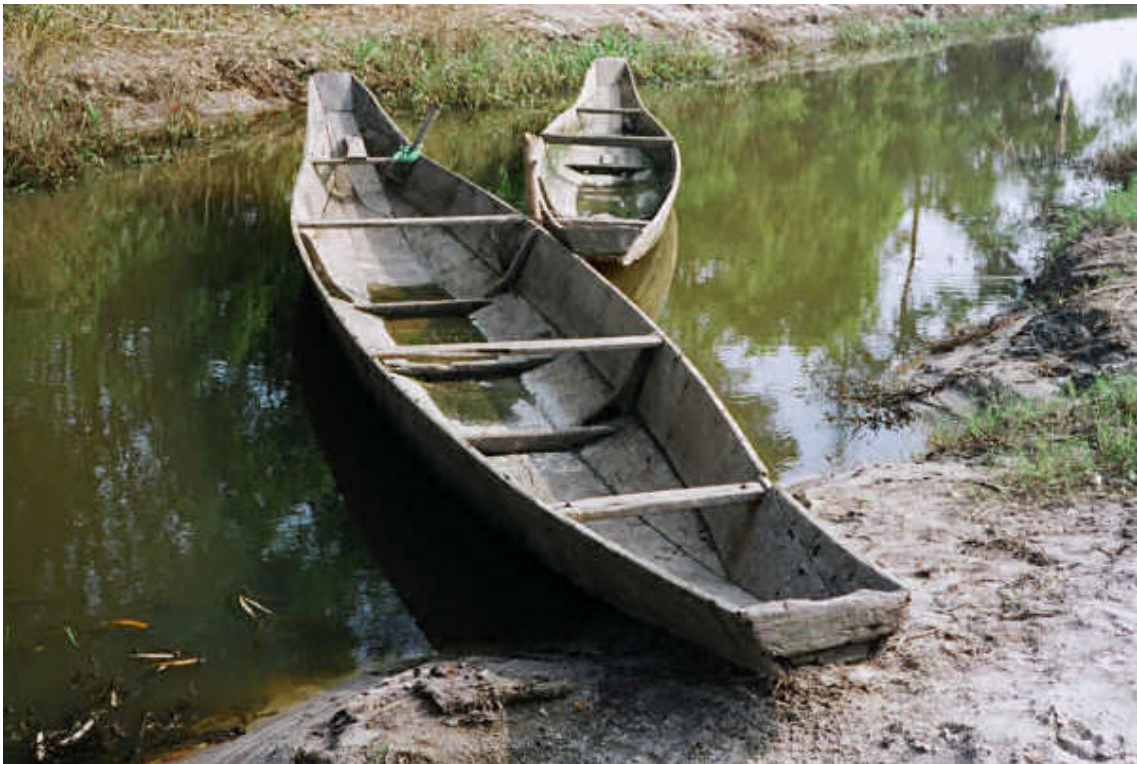
Figure 49: Plank boat: Typical Vietnamese Five- plank boat from Central coast and Ron river. Boat is flat bottomed, with shovel ends, flaring sides, and quite long for their width. (Photography: Ken Preston [On line] Available at: < http://www.boatsandrice.com/cVN.html > [29. May 2015]).
