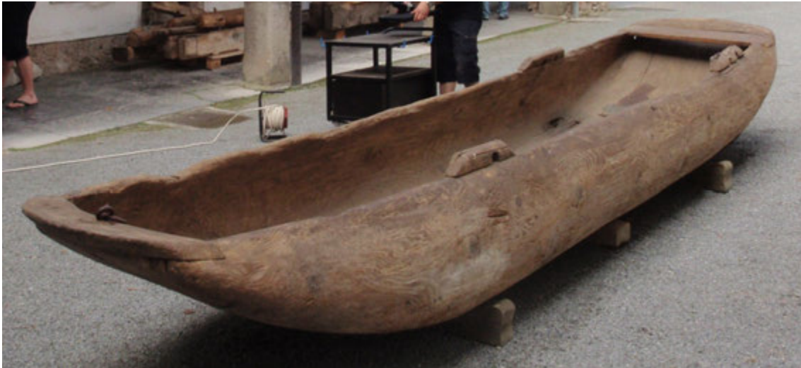
Figure 22: Logboat: Special autochthonous construction of multi- extended logboat caled drevak which mean tree- boat, isolated in Notranjska region, Slovenia, perhaps with the roots in Roman period. It is made from fir with two part of logboat as chine-girders with one or two inserted bottom planks. Exposed in Technical Museum of Slovenia, Bistra (Photography: Miran Erič).
