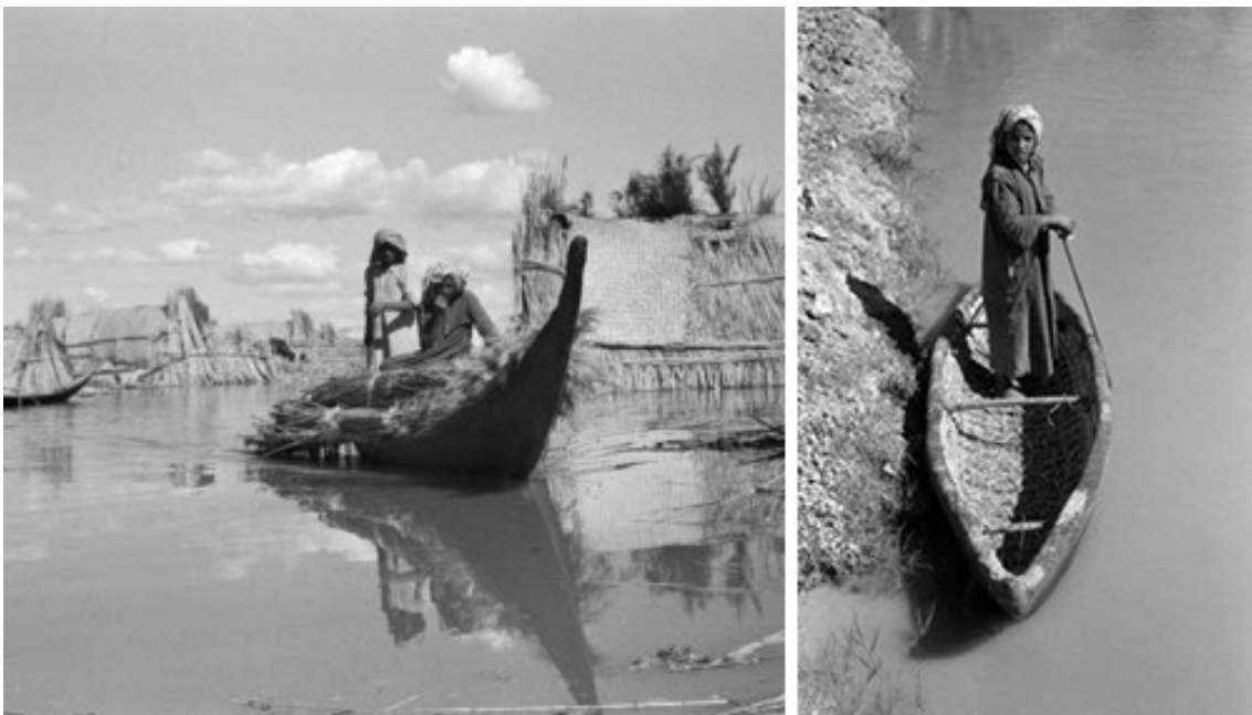
Figure 38: Reed boat: Zaima is an typical Al Hasans people woven phragmites grass basket double ended boat from Karmashiya in Hawizeh Ma'dan or Marche Arab in Iraq. Preparation of dry phragmites reeds for use in boat and house building on left and form of typical boat (Photography: Wilfred Patrick Thesiger [On line] Available at: < https://www.pinterest.com/pin/350928995939783941/ > [29. May 2015]).
