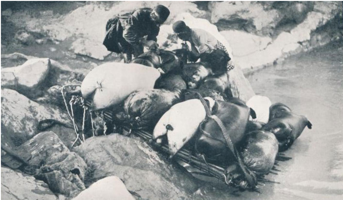
Figure 13: Skin boat: Goat Skin Raft is basically made from 9 to 15 inflated, goat, lamb, or other similar inflated animal skin bound to each other with light wooden platform. This raft, photography taken in 1927, is from Karoun, Bakhtiari mountain, Bakhtiari province, Iran (Photography: Viktoria Mary Sackville-West; Anglo- Persian Oil Company [On line] Available at: http://www.gutenberg.ca/ebooks/sackvillewest-twelvedays/sackvillewest-twelvedays-00-h-dir/sackvillewest-twelvedays-00-h.html#img-119 ) [29. May 2015])
