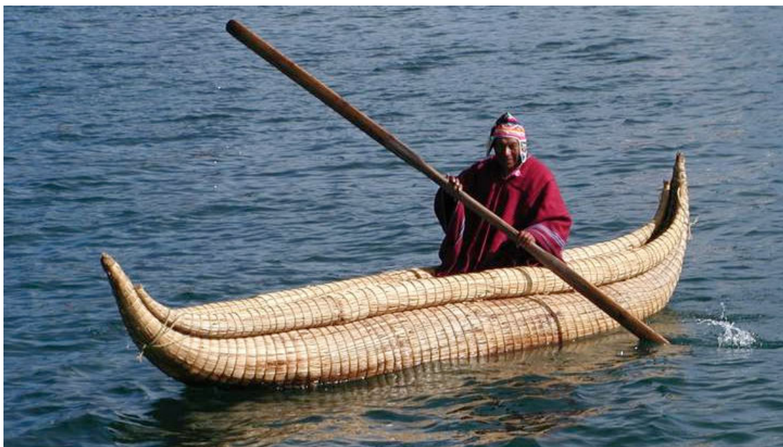
Figure 33: Reed boat: Lake Titicaca between Peru and Bolivia is one of the most known areas in the world where reed boats are still part of the everyday lives of the locals. The boats are all named balsa and vary in size from small to as large as 30m long. Typical totora bullrush small canoe-like boat from the Lake. (Photography: Andre Engels [On line] Available at: < https://en.wikipedia.org/wiki/Reed_boat > [29. May 2015]).
