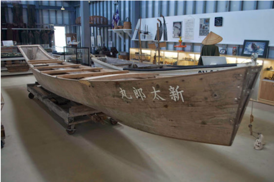
Figure 50: Plank boat: Typical plank boat sabani from fishing port Itoman in Okinawa. Boat is "V" formed chine and fastened with hardwood butterfly keys huundu (Photography: Douglas Brooks [On line] Available at: < http://blog.douglasbrooksboatbuilding.com/2014/07/okinawa.html > [29. May 2015]).
