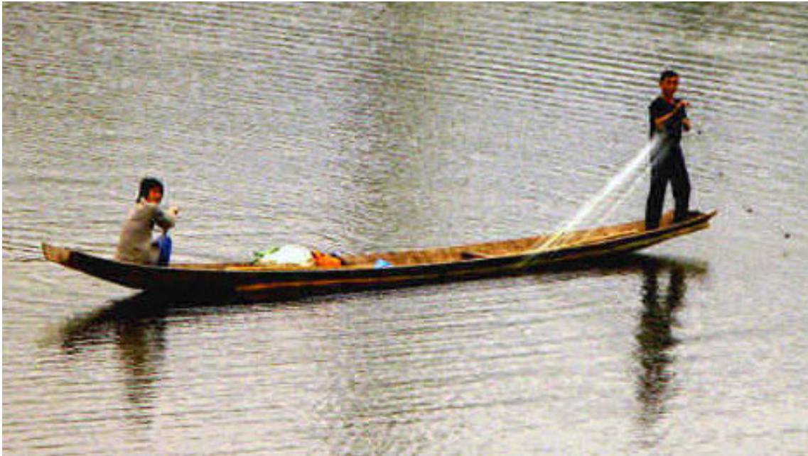
Figure 48: Plank boat: Typical Three- plank boat sampan from Mekong river in Laos. Boat is flat bottomed, with shovel ends, flaring sides, and quite long for their width. It is joined and stitched with rattan or bamboo strips, which in later times were replaced by bamboo nails or iron nails. A further improvement was the use of tenoning. (Photography: Ken Preston [On line] Available at: < http://www.boatsandrice.com/Lmekong.html > [29. May 2015]).
