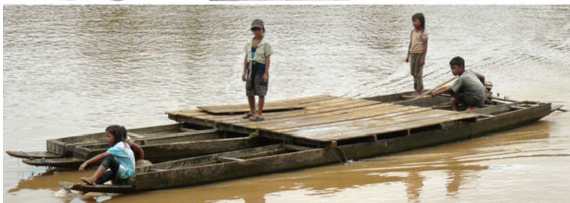
Figure 27: Logboat: Typical paired logboat from Bug river northern part of Poland with special Polish name komjagami , now placed in Sadowne Museum, top (Waldemar Ossowski, Studia nad Lodziami jednopiennymi z obszaru Polski , Prace Centralnego Muzeum Morskiego w Gdansk, tom XI 1999, p. 156, figure 140) Modern use of multi-hulled boat made with three logboats from Xekong River in Laos bottom (Photography: Ben Visbeek [On line] Available at: < https://www.flickr.com/photos/81035653\spacefactor/@mN00/4414226741 > [29. May 2015]).
