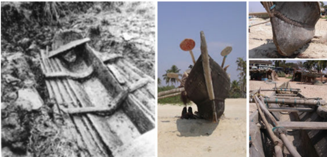
Figure 23: Logboat: Left Type of typical European 13 rd century extended logboat with side planks coupled with the ribs from Kentmere, Cumbria discovered by David G. Wilson. (Photography: David Wilson; Seán McGrail, Ancient Boats in North-West Europe. The Archaeology of Water Transport to AD 1500 , Longman AS 1998, p. 75, figure 6.15). Right Typical extended modern logboat use in Goa, India with high exposed constructional solution. Today extended logboats are often in combination with outriggers logboats specially for using on seas (Photography: Paul Wilson, Archive of Indigenous boat blog site of Bob Holtzman [On line] Available at: < http://counter-agency24.rssing.com/chan-12927004/all_p1.html > [29. May 2015]).
