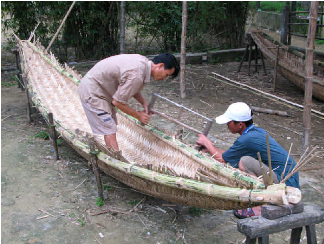
Figure 37: Reed boat: Typical Vietnamese thung-chai woven bamboo basket double ended boat from Da Nang region. (Photography: Ken Preston [On line] Available at: < http://www.boatsandrice.com/wovenBamboo.html > [29. May 2015]).
