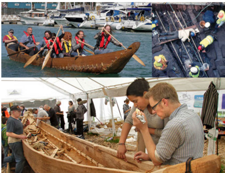
Figure 47: Plank boat: Dover boat was constructed of oak planks, stitched together with yew withies and also fixed together with wooden wedges (Top left: Paddling a half scale replica, top right: Excavation in 1992 and bottom: Replica reconstructing 2013 [On line] Available at: < http://www.canterburytrust.co.uk/trust-blog/ > [29. May 2015]).
