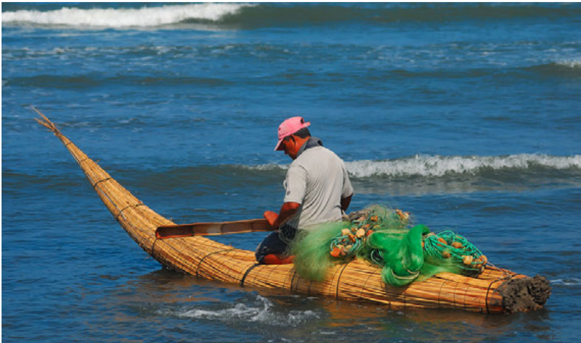
Figure 32: Reed boat: Typical tutora boat called cabalito del totora or horse reed boat from the Trojiljo district on northern Pacific coast of Peru. Coastal fishing. (Photography: Martin Garcia [On line] Available at: < https://www.flickr.com/photos/martix/4321613099 > [29. May 2015]).
