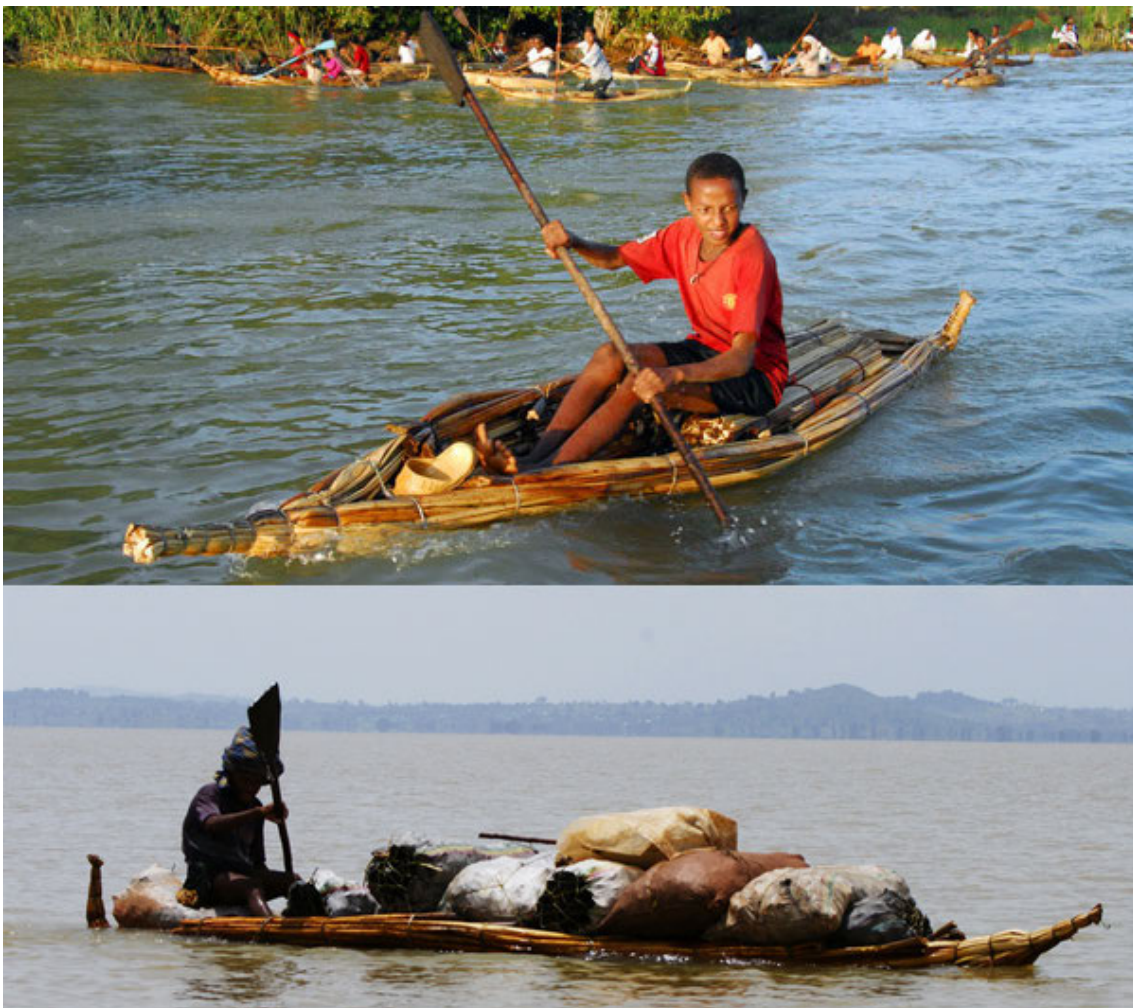
Figure 30: Reed boat: very simple kayak-like shaped Tankawa papyrus boat paddled by two bladed paddle on Lake Tana, Ethiopia (Photography top: Brian J. McMorrow [On line] Available at: < http://www.pbase.com/image/108955080 >) (Photography bottom: "Djib" by Flickr [On line] Available at: < https://www.flickr.com/photos/99631178\spacefactor\@mN00/2645782736 > [29. May 2015]).
