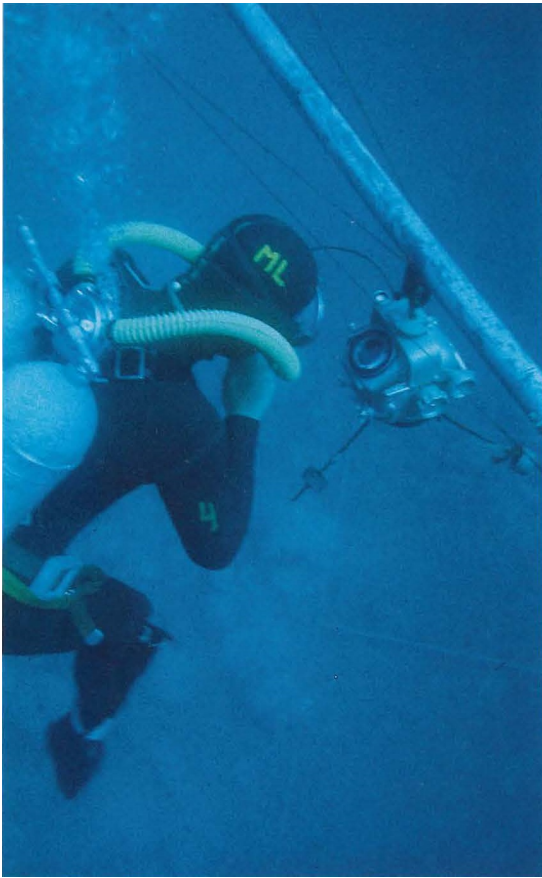
Above Donald Rosencrantz slides a camera, hanging vertically on gimbals, along a horizontal bar above the 7th-century Byzantine shipwreck at Yassıada, Turkey. He takes pictures at predetermined points marked on the bar, providing pairs of stereo photographs from which accurate three-dimensional plans can be made.
