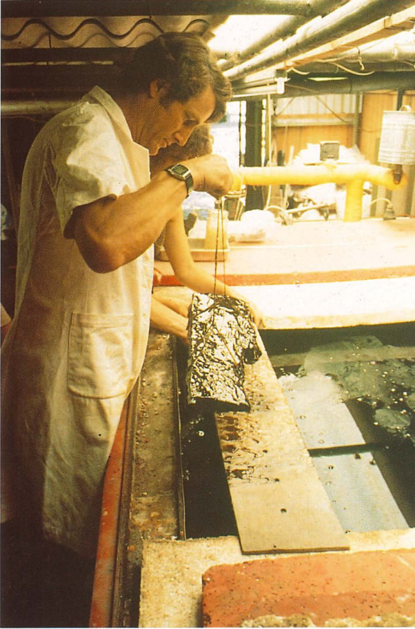
Soaking wood in polyethylene glycol.
