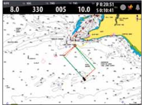
Laylines calculated from True Wind Angle displayed on a Chartplotter
