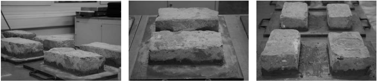
Figure 1. Old, solid bricks used for shear tests.
