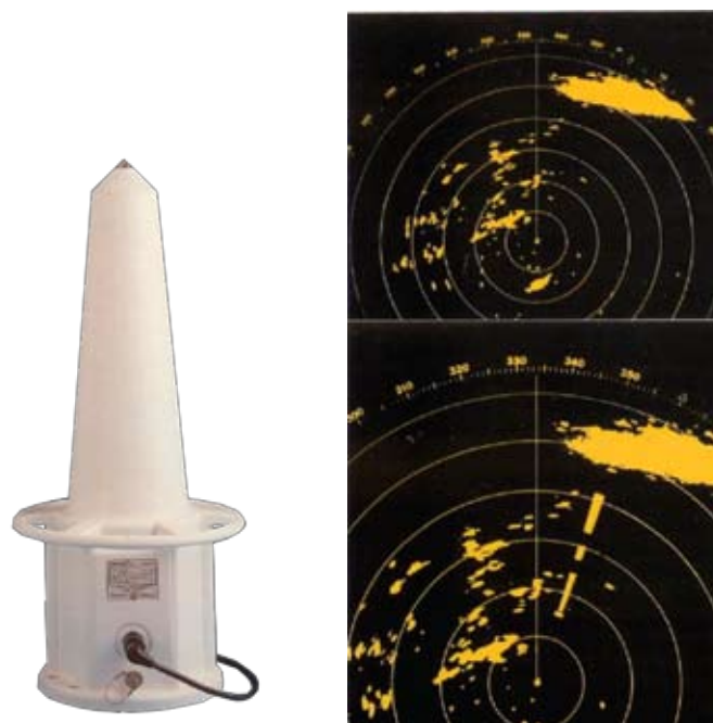
Figure 18 – Example of a racon and a radar display with and without the racon character
