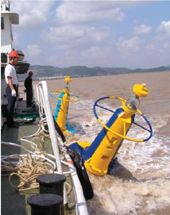
Synthetic buoy (Emergency Wreck Mark) Photo courtesy of China Maritime Safety Administration
