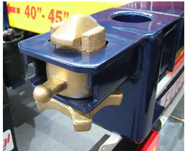
Twist-lock on a rear corner of a container semi-trailer; the container corner is placed over it and has to be turned 90° to close the lock (picture Wikipedia).
