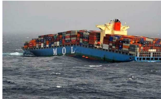
MOL Comfort (316 m long) broken in two parts during a storm in the Indian Ocean and sunk in June 2013 (picture http://www.meretmarine.com ).
