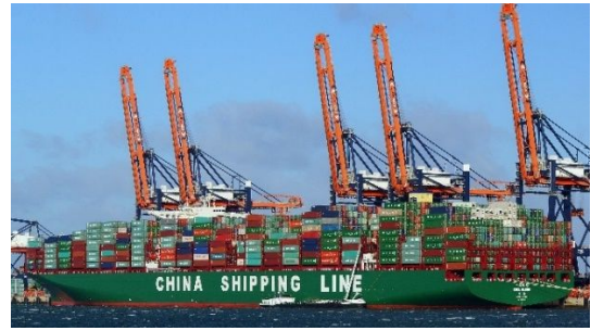
Five gantry cranes with lifted arm allowing ship movement. Such a berth can move around 150 TEU per hour (picture https://www.marinetraffic.com ).
