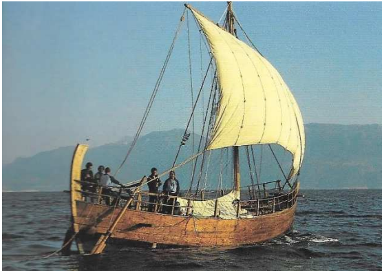
Kyrenia II (3 rd c. BC) sailing at close reach with a square sail on the Aegean Sea in 1987 44 (picture Pomey, 1997).
