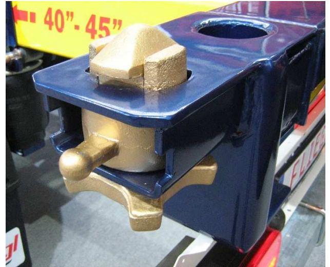
Twist-lock on a rear corner of a container semi-trailer; the container corner is placed over it and to close the lock, it has to be turned 90° (picture Wikipedia).
