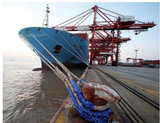
Five gantry cranes with lifted arm allowing ship movement. Such a berth can move around 150 TEU per hour (picture https://www.marinetraffic.com ).
