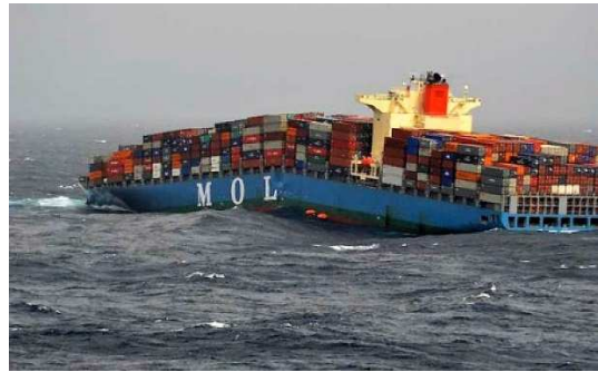
MOL Comfort (316 m long) broken in two parts during a storm in the Indian Ocean and sunk in June 2013 (picture http://www.meretmarine.com ).
