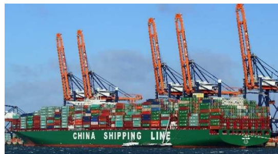
Five gantry cranes with lifted arm allowing ship movement. Such a berth can move around 150 TEU per hour (picture https://www.marinetraffic.com ).
