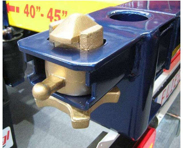
Twist-lock on a rear corner of a container semi-trailer; the container corner is placed over it and to close the lock, it has to be turned 90°(Wikipedia).
