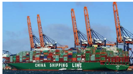
Five gantry cranes with lifted arm allowing ship movement. In order to save time, even more gantry cranes are sometimes used (picture https://www.marinetraffic.com ).
