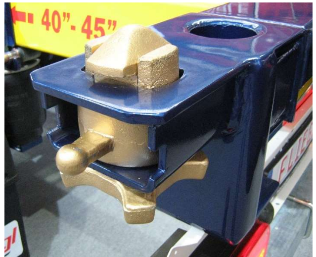
Twist-lock on a rear corner of a container semi-trailer; the container corner is placed over it and it has to be turned 90° to close the lock (picture Wikipedia).
