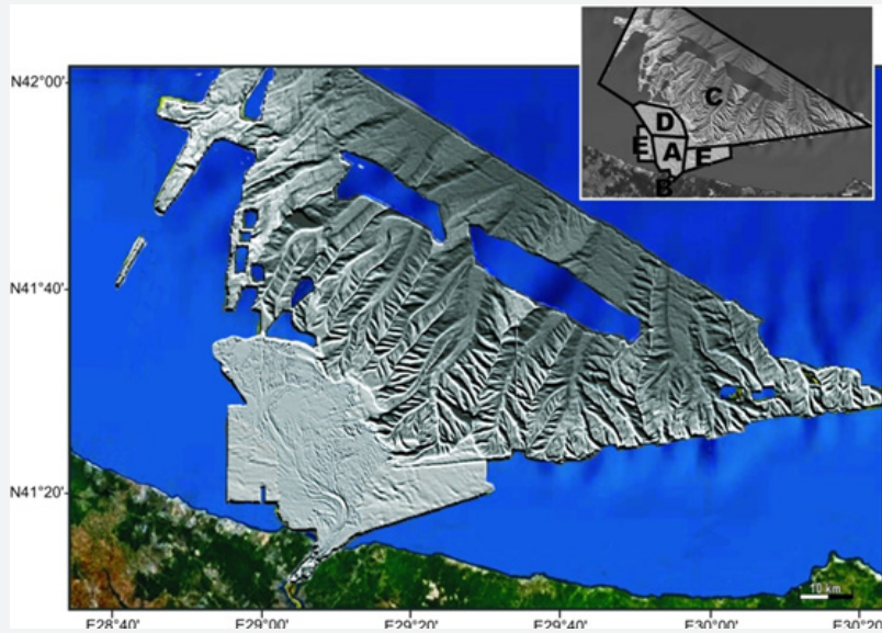
Figure 1: Multibeam bathymetric map of the South-Western Black Sea presenting the studied shelf fan. Synthesis was realized with data issued from:
