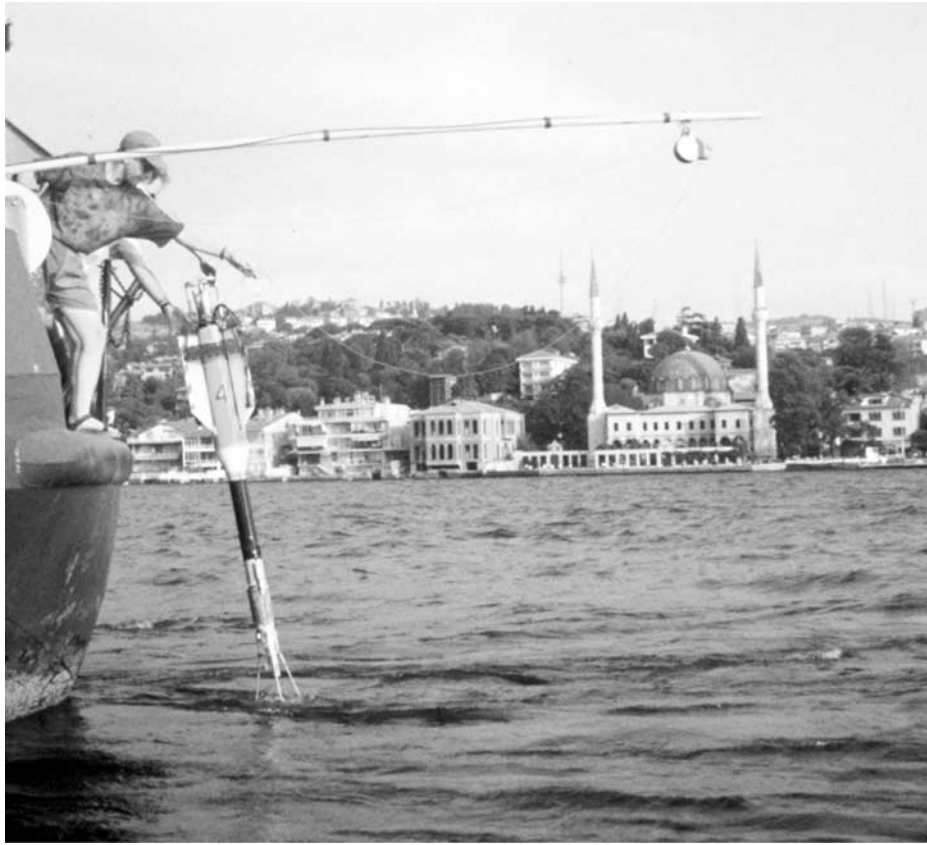
Figure 2. Launching an AMP in the southern Bosphorus, about 8 km from the Marmara entrance and looking toward the Asian side, which rises steeply behind a narrow beach. A probe guard was mounted on the bottom of the instrument to permit landing on the bottom. The thin blue tether transmitted data via a fiber-optic cable inside a Kevlar jacket for strength. The tether passed through a pulley mounted on the end of a fiberglass pole. The stiff, but flexible, pole damped sudden jerks on the line during recovery.
