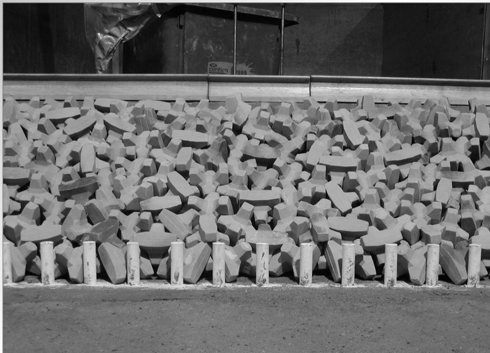
**Figure 6.20** View of the model test for typical toe detail using concrete piles (courtesy HR Wallingford)
