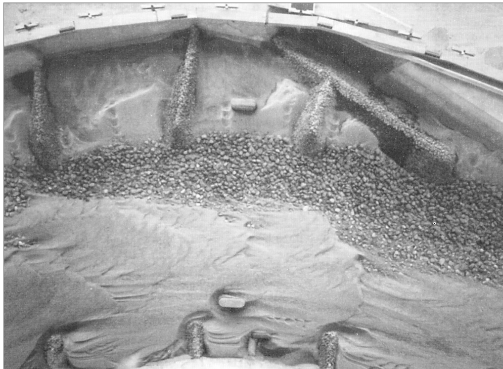
Figure 4.91 Example of a physical model of a river with mobile bed (courtesy WL|Delft Hydraulics)
