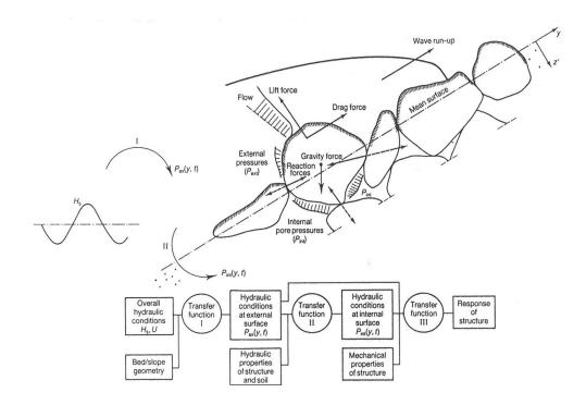
Figure 2.2 A rock system and its responses to hydraulic loading (waves)
