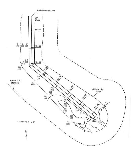
Figure 10.8 Contours of equal settlement or displacement of armourstone on a breakwater (Weymouth and Magoon, 1969)
