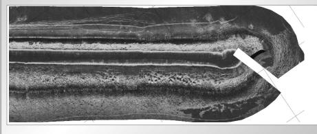
Figure 10.13 Multi-beam image of Peterhead Breakwater (courtesy EMU Environmental)
