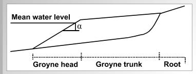
Figure 10.19 Longitudinal section of a groyne
