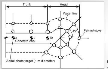
Figure 10.7 Armour survey scheme
