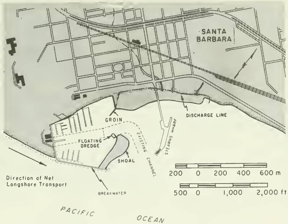
Figure 6-47. Sand bypassing, Santa Barbara, California.
