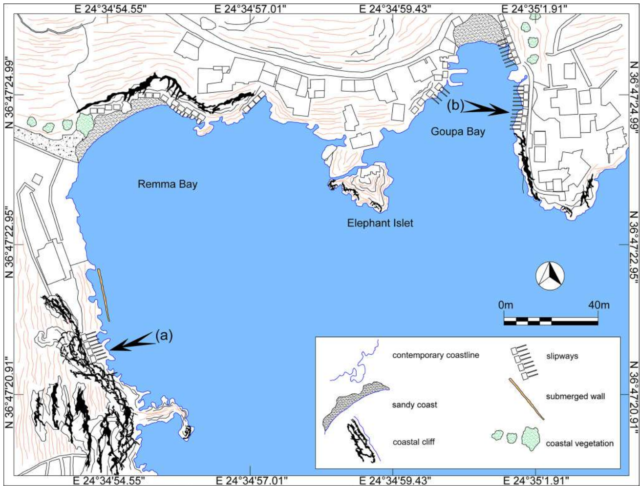
Fig. 22 Location map of Remma and Goupa Bays. Arrows a , b indicate the slipways that are presented in the cross-sections of Fig. 23
