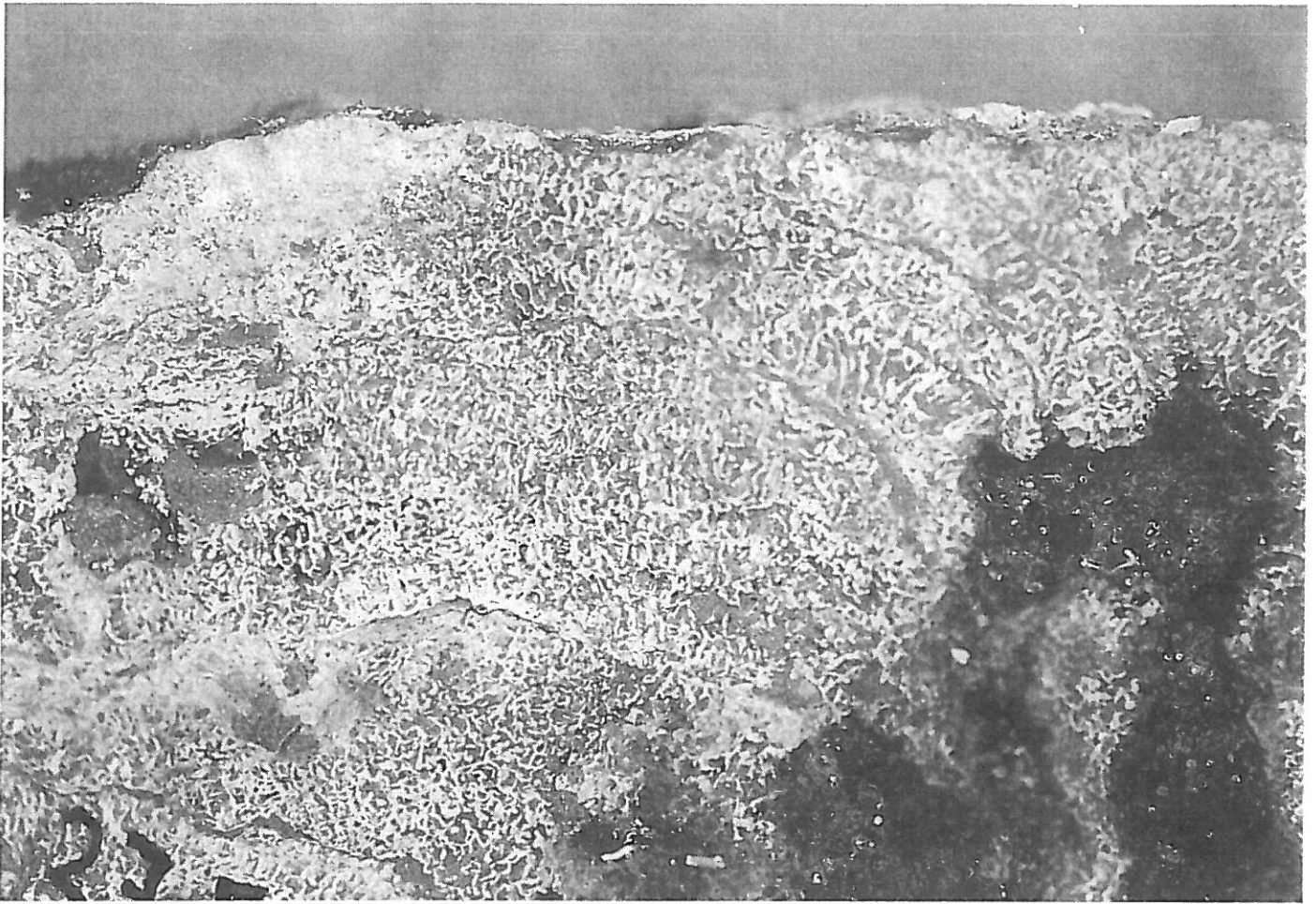
Fig. 11. Section through the present rim at La Ciotat. Algal thalli appear in white and cemented areas in brown. Several horizontally superposed layers of hardened thalli are also visible. The length of the specimen is about 20 cm.
