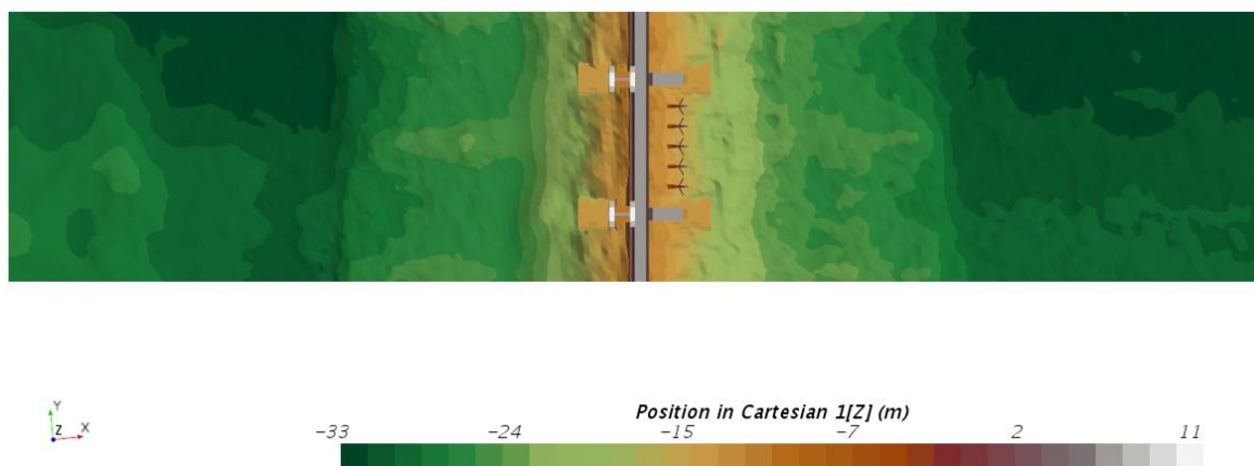
Figure 3.10 Contour plot of the bed elevation. Dimensions are with reference to NAP.
