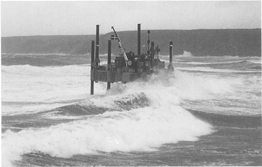
Figure 5.1. Wave loads on walking jack-up platform (courtesy Seacore Ltd)
