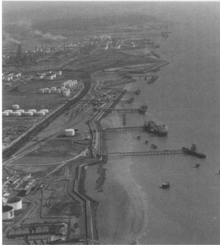
Figure 7.5. Shellhaven Refinery. Relatively sheltered environment where peak currents are typical 1–1.5 m/s (courtesy Costain)
