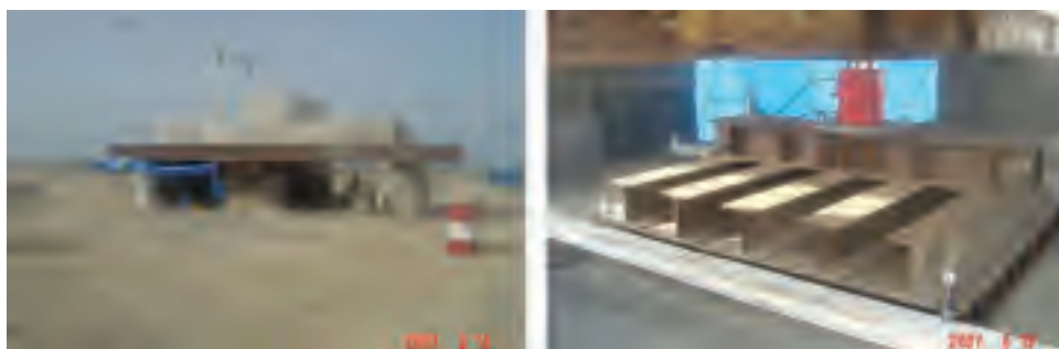
Figure B.43 Arrangement for a Zone Load Test.
