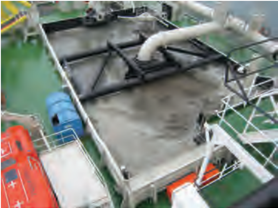
Figure A.13 Overflow on board a trailing suction hopper dredger.
