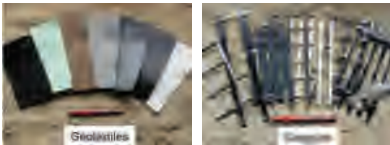
Figure 8.33 Geotextile and geogrid.
