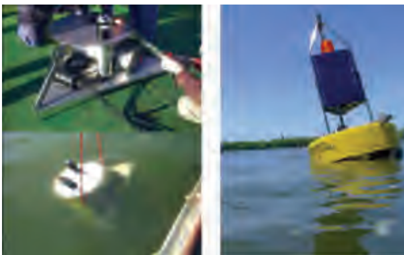
Figure B.51 Seabed installed frame and monitoring buoy [Ref. http://www.osil.co.uk , http://www.ysi.com ].
