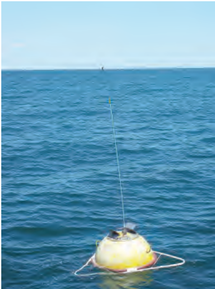
Figure B.32 Directional wave rider buoy (Datawell).
