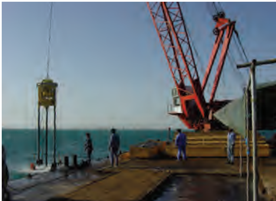
Figure B.13 Deployment of a vibrocorer.
