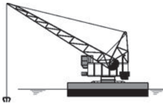
Figure 4.6 Grab dredger with a wire suspended grab installed on a pontoon.
