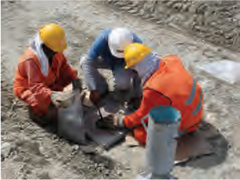
Figure B.25 Performing the Sand Cone Test.
