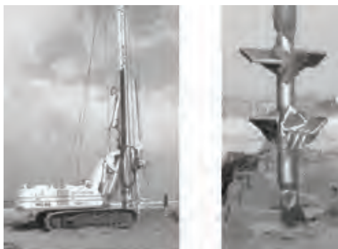
Figure 7.26 Deep soil mixing equipment (Moseley et al. , 2004).
