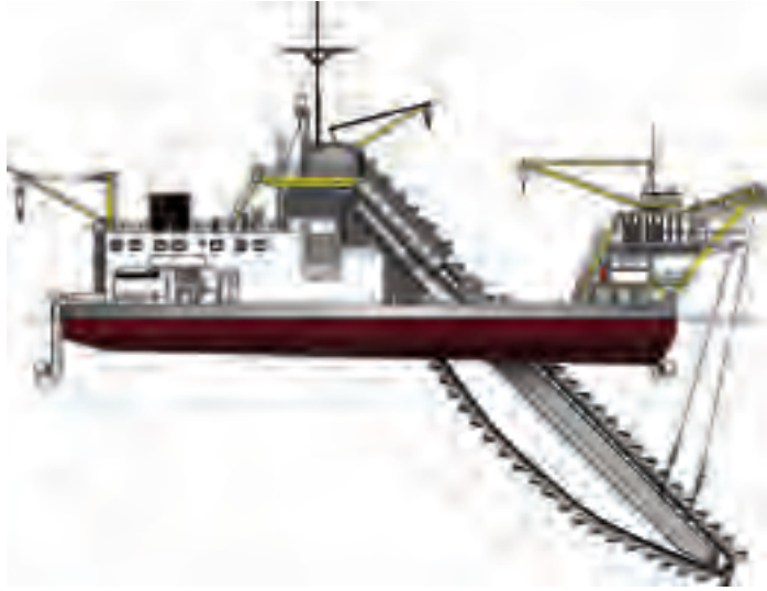
Figure A.25 Bucket dredger with a raised ladder.
