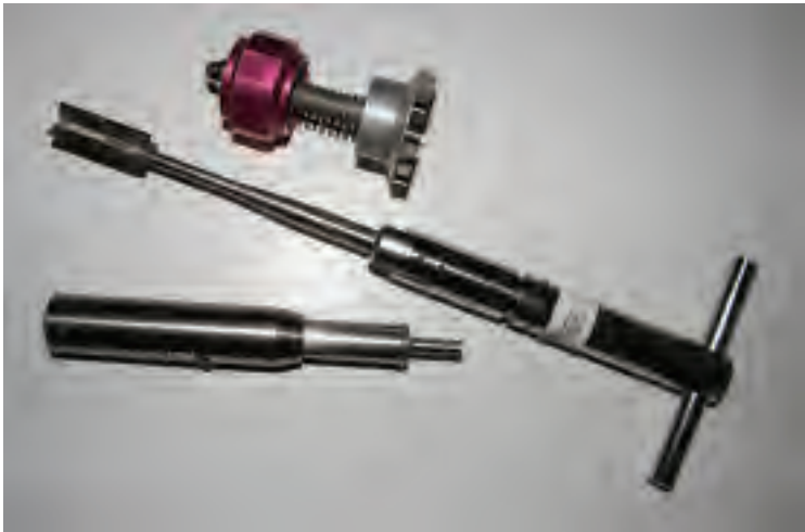
Figure B.22 Field equipment hand vane and pocket penetrometer.
