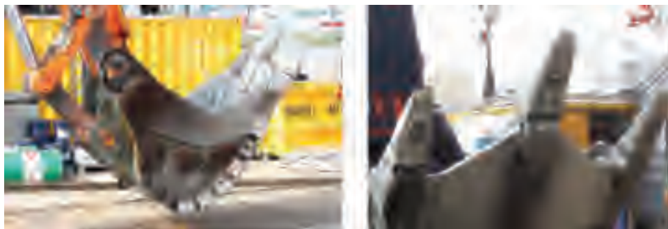
Figure A.20 Backhoe bucket for dredging in hard material.
