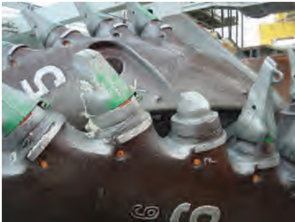
Figure 9.37 Wear and tear to cutter head during rock dredging.
