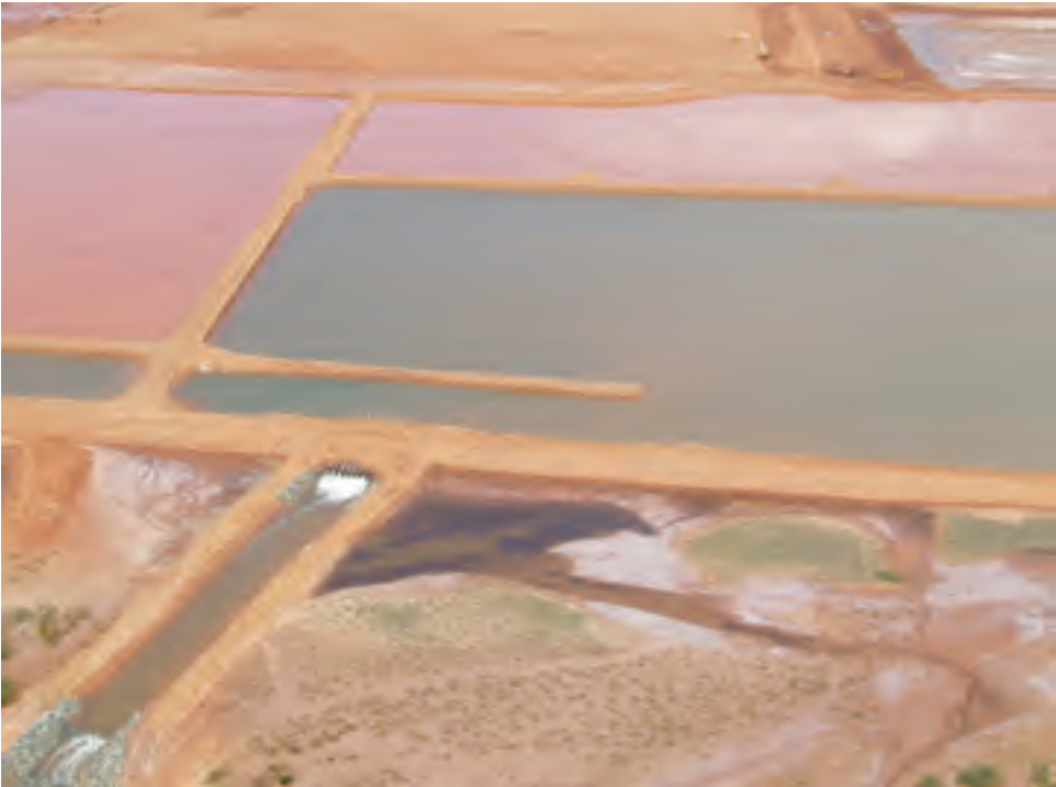
Figure 6.18 Example of settling pond lay-out.
