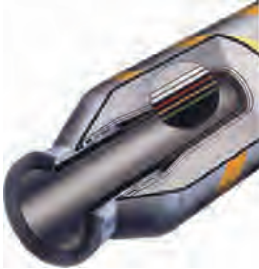
Figure A.32 Floating pipe line of reinforced rubber.
