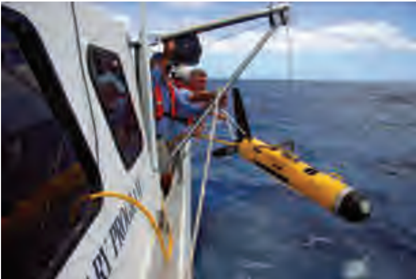
Figure B.37 Retrieving a side scan sonar device (Photo: NOAA).
