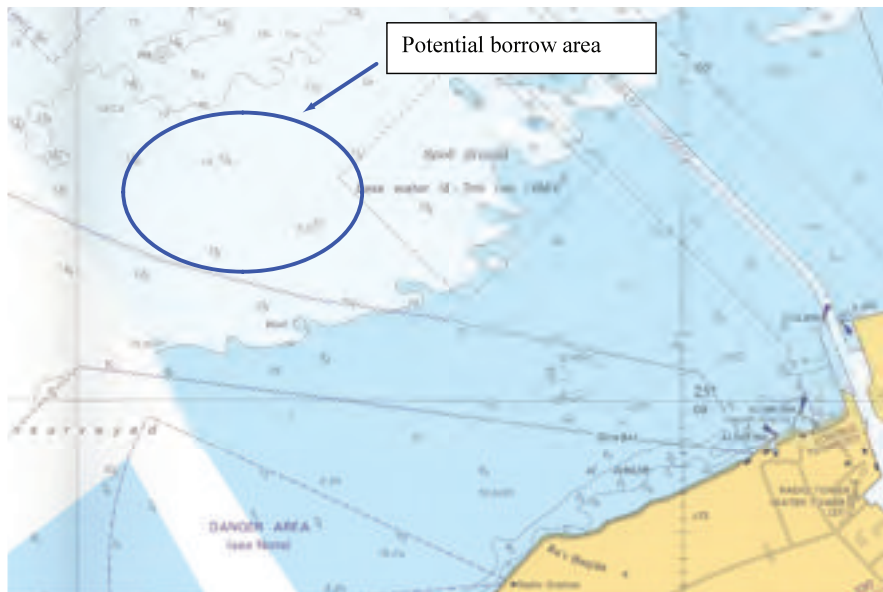
Figure 3.5 Definition of a potential borrow area based on information on an admiralty chart (location: Dubai).
