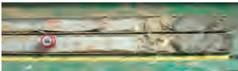
Figure 3.8 Torvane test on vibrocore sample.
