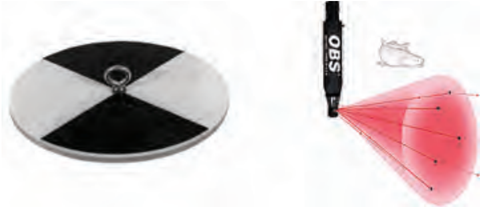
Figure B.36 Example Secchi disk (ref www.geoscientific.com ) and turbidity meter.
