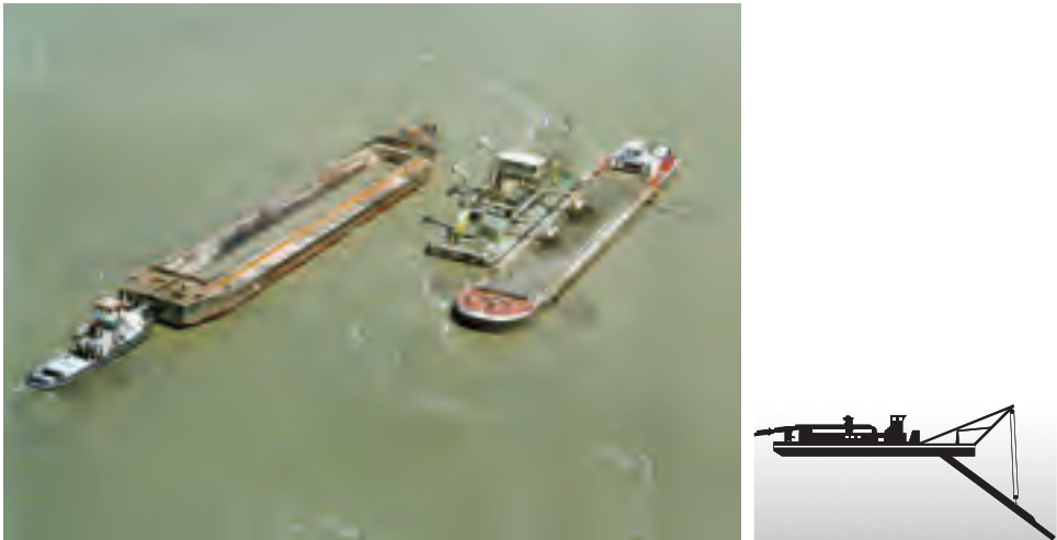
Figure 4.2 Plain suction dredger loading barges.
