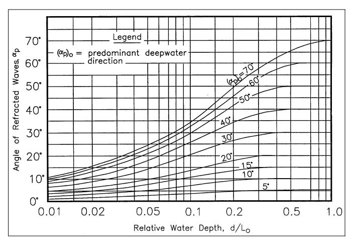
Figure 3-20. Variation of predominant wave direction for random sea waves on a coast with straight and parallel bottom contours (Goda 1985)
