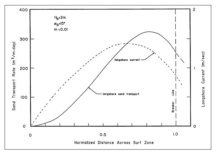
Figure 6-7. Calculated cross-shore distribution of longshore transport
