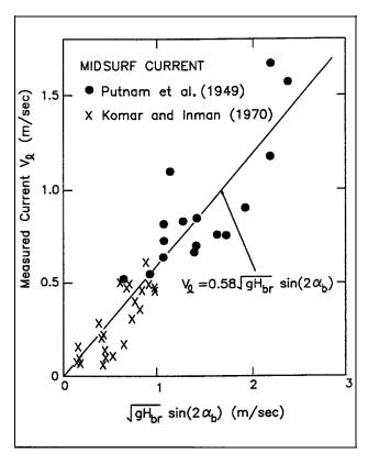
Figure 5-2. Field measurements of longshore current
