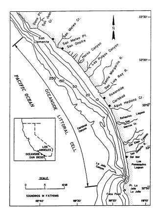
Figure 7-4. Oceanside littoral cell
