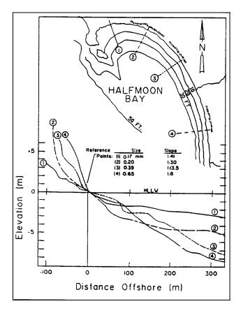
Figure 4-3. Systematic changes in the beach face slope along the length of Halfmoon Bay, California (after Bascom 1951)
