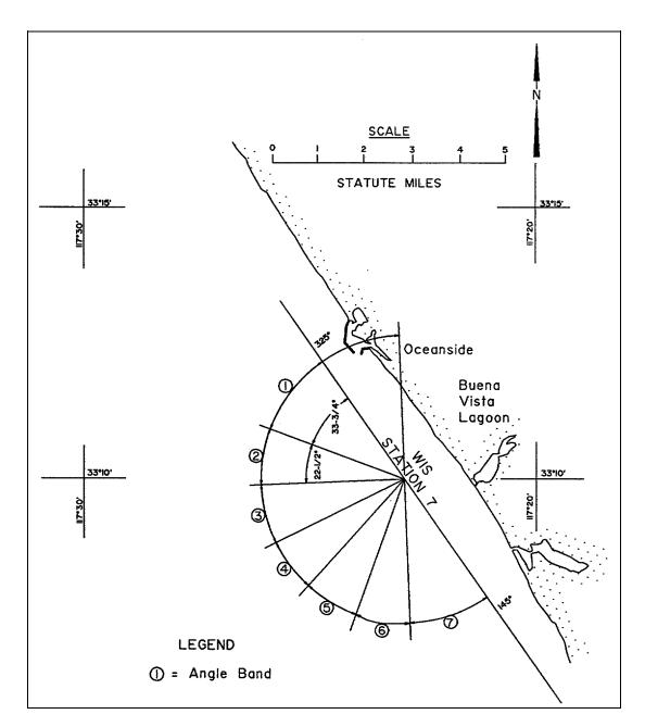
Figure 7-7. Orientation of wave angle bands at Oceanside
