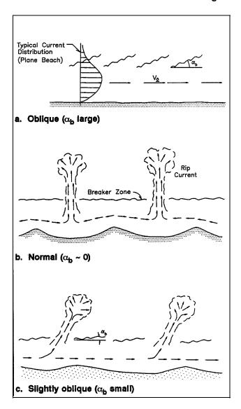
Figure 5-1. Observed horizontal circulation patterns as a function of wave approach
