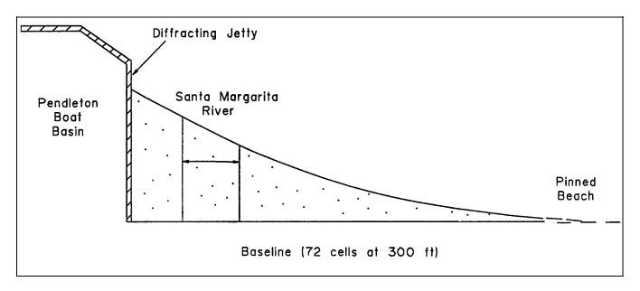
Figure 7-8. Idealized features of Oceanside north reach
