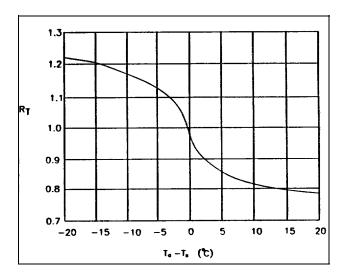
Figure 3-14. Correction factor for the air-sea temperature difference,  $(T_a - T_s)^{\circ}C$  (after Resio and Vincent 1977)
