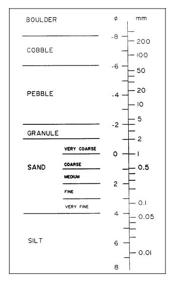
Figure 4-1. Wentworth and  $\phi$  grain size scales
