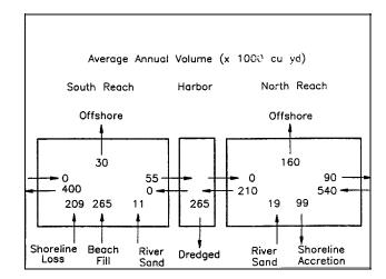
Figure 7-12. Sediment budget for Oceanside
