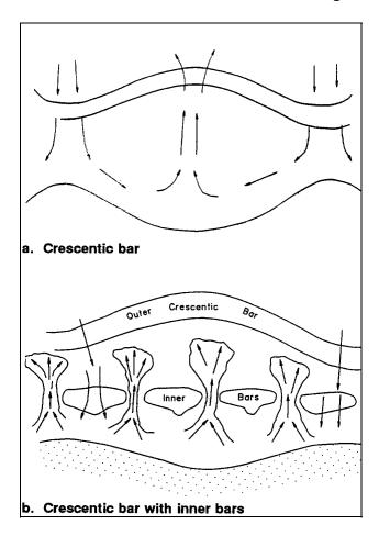
Figure 2-3. Cell circulation patterns due to various morphologies
