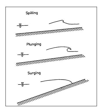
Figure 3-23. Breaking wave profiles
