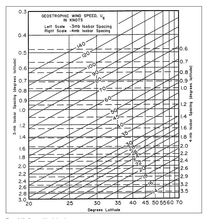
Figure 3-13. Geostrophic wind scale
