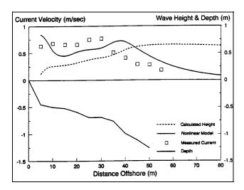
Figure 5-3. Example NMLONG simulation for multiple barred beach
