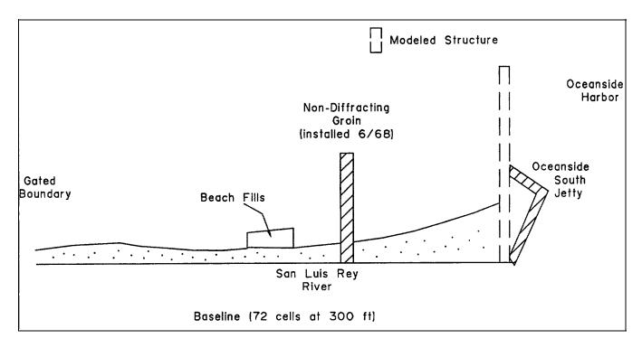
Figure 7-9. Idealized features of Oceanside south reach
