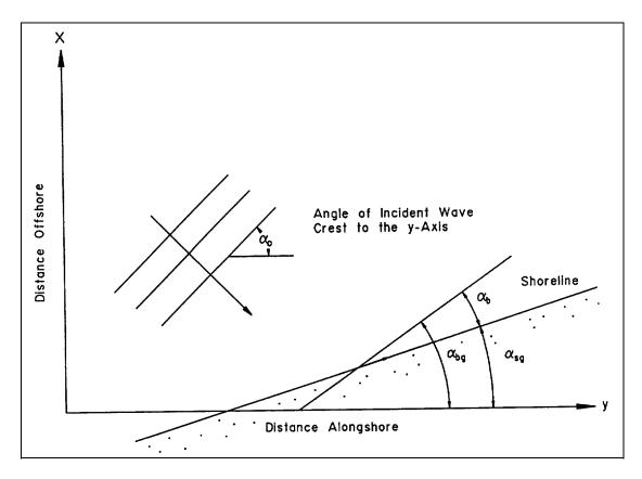
Figure 6-9. Definition of local breaker angle
