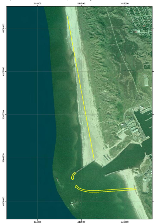
Figure 5: Proposed future layout of Hvide Sande Harbour breakwaters (curved yellow lines). The shoreline location after the beach excavation north of the harbour is illustrated by a straight yellow line, which also indicates the extent of the proposed dredging
