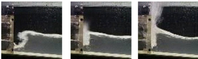
Fig. 16.4. An impulsive (breaking) wave at a vertical wall, resulting in an impulsive (violent) overtopping condition.
