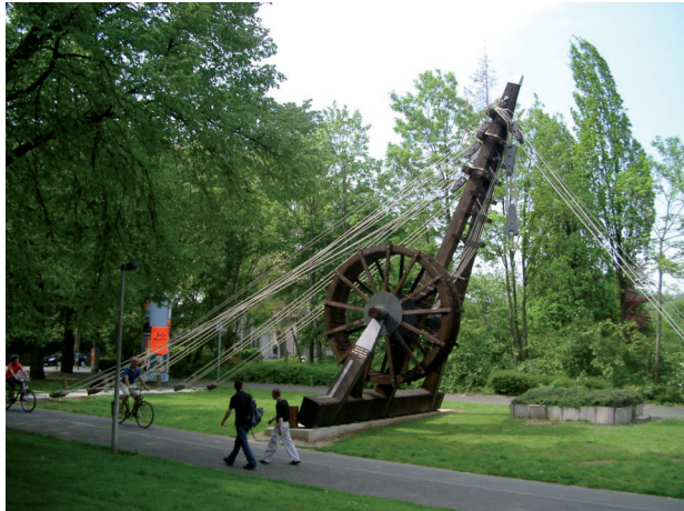
Figure 4.1: Replica of Roman treadmill powered crane, replica Bonn [Wikipedia]
