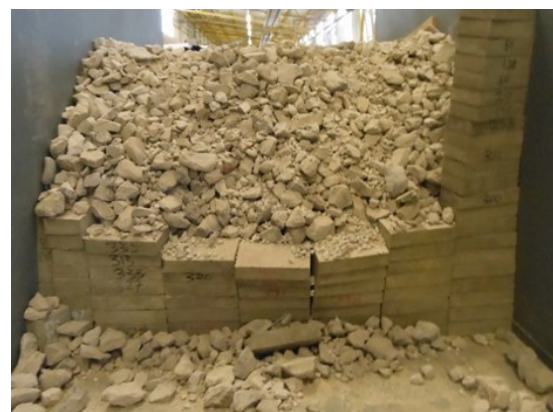
Figure 4: Failed dry-build. Left - immediately after collapse. Right - failed structure with spilled core removed to reveal arched (but still intact) wall toe.
