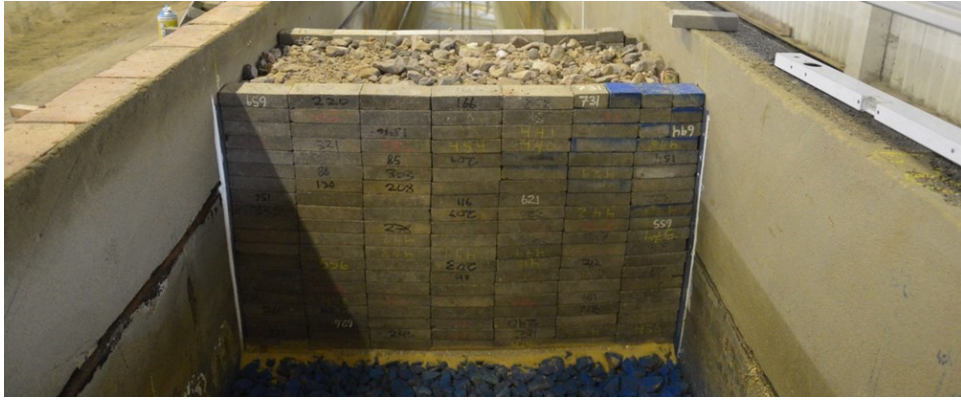
Figure 6: Example test structure in flume.
