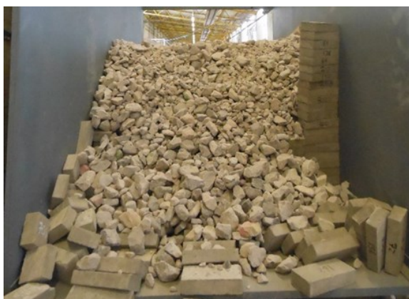
Figure 4: Failed dry-build. Left - immediately after collapse. Right - failed structure with spilled core removed to reveal arched (but still intact) wall toe.
