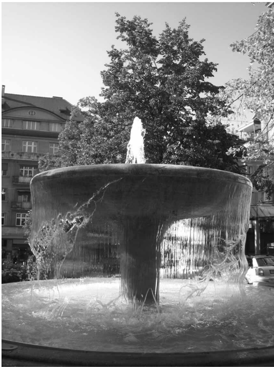
Figure 3 Surface tension effects in water fountain at Rämistrasse, Zurich, resulting in separation of water sheet (Photo V. Heller)
