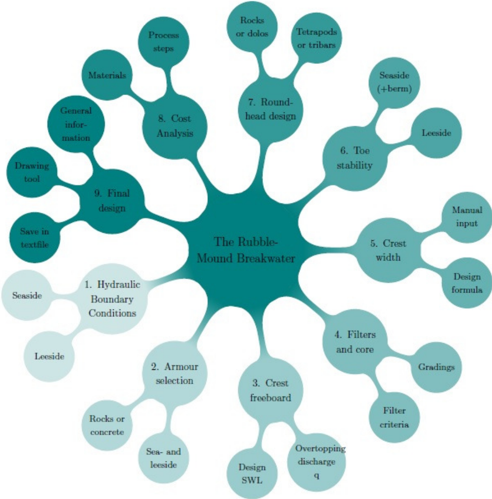
Figure 7: Design steps for the rubble-mound breakwater
