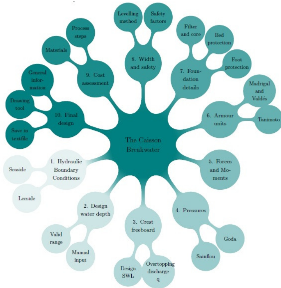
Figure 47: Design steps for the caisson breakwater
